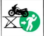
Maintain a safe distance from lift if there is a possibility of the motorcycle falling down. Failure to do so may result in physical danger or death.
